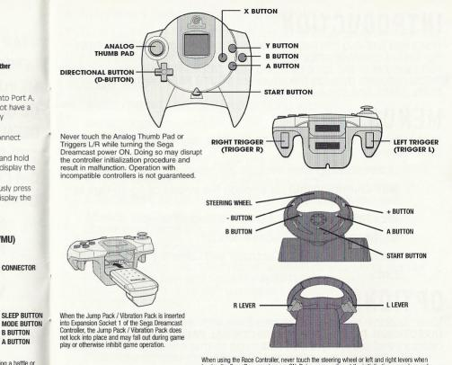
turning the Sega Dreamcast power ON. Doing so may disrupt the initialization procedure and result in malfunction if readiustment is not properly carried out via the Options menu. If the handle or levers are accidentally moved while turning the power ON, immediately turn the power OFF and ON again making sure not to touch the Race Controller.
